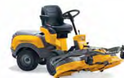
The Combi deck can be raised 30 degrees for cleaning without having to remove the belt (Park 4WD only).
