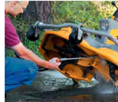
Service and wash friendly design. The Combi deck can be raised 30° for cleaning without removing the belt.
