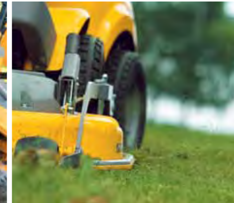
Front mounted cutting deck goes anywhere. Note the reinforced frame that protects against knocks and also acts as a lifting handle.
